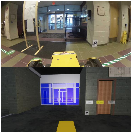
Figure 6 The robot in the job site (top), and the 3D virtual environment (bottom) visualized in real-time simultaneously
